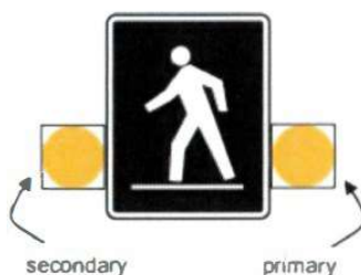
FIGURE 9: SPECIAL CROSSWALK ASSEMBLY
