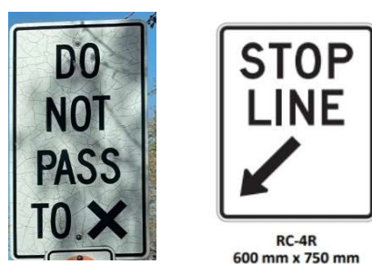
FIGURE 12: SUBSTANDARD AND STANDARD RC-4 STOP LINE SIGNS
