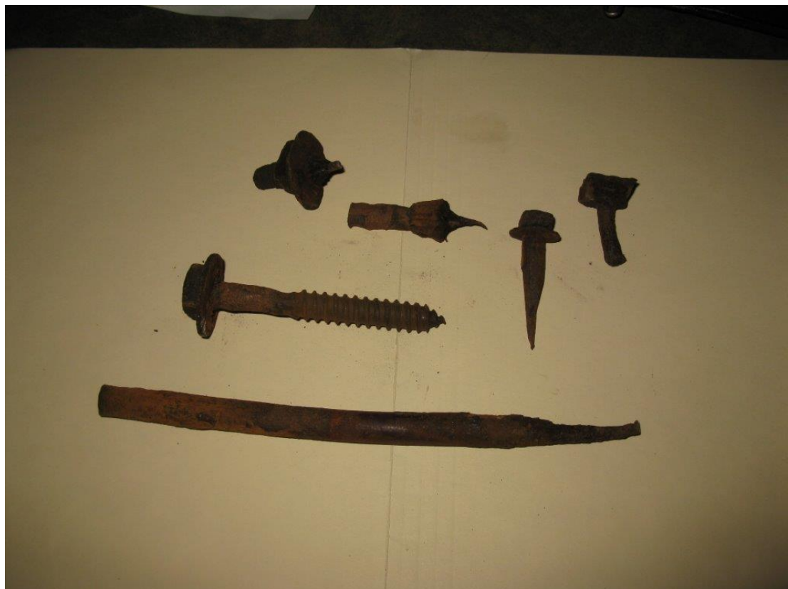
Example of Badly Corroded Bell Support Bolts
